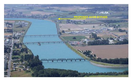
The photo above is a conceptual view of the Skagit River looking westerly with the Avon Bend in the distance. In this view, levees have re-located to provide a wider river channel and the proposed Avon Bypass is shown in the distance.
