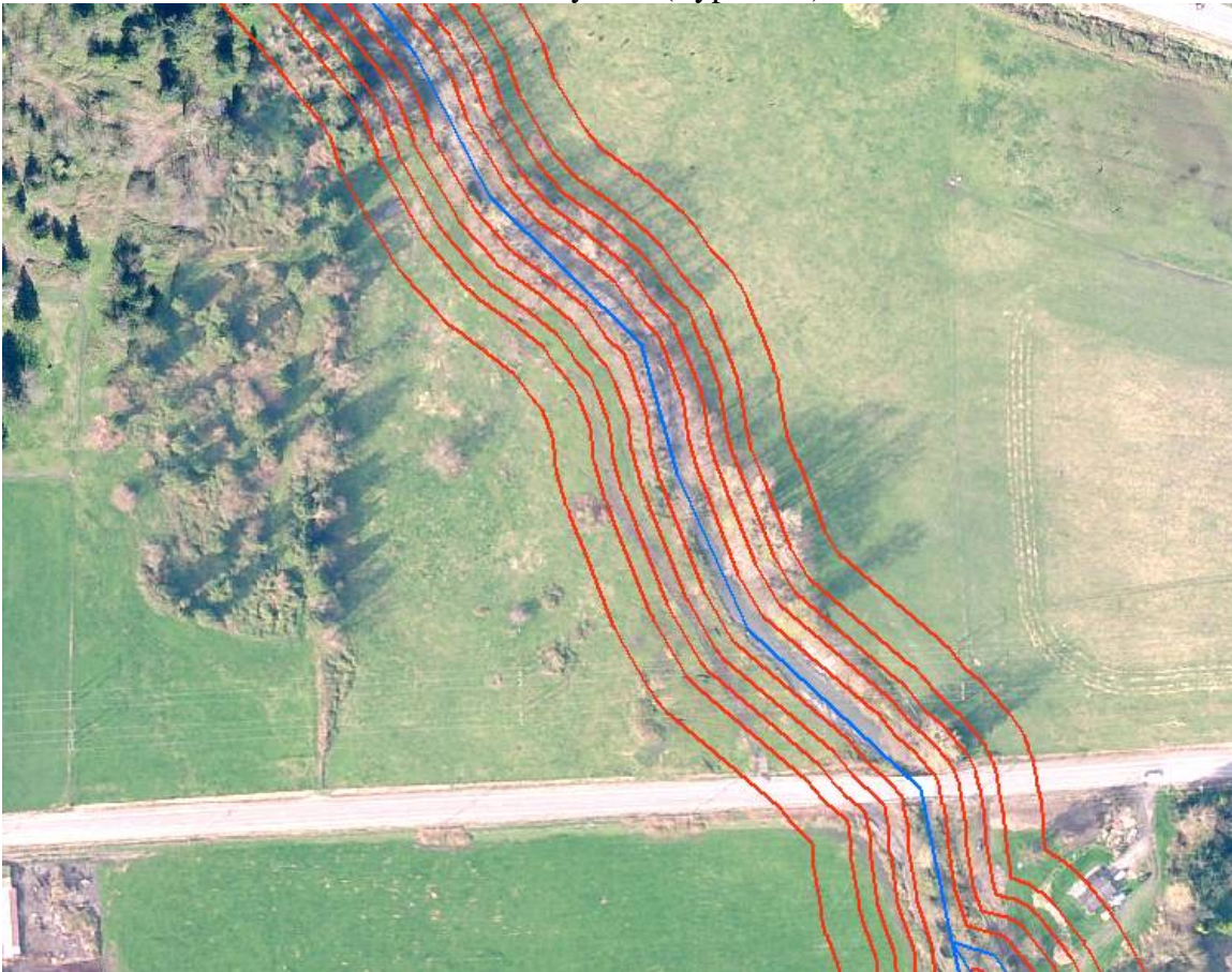
Figure 25. Example of multiple buffer distances around a single watercourse to assess how land cover changes with increasing distance from the watercourse.
