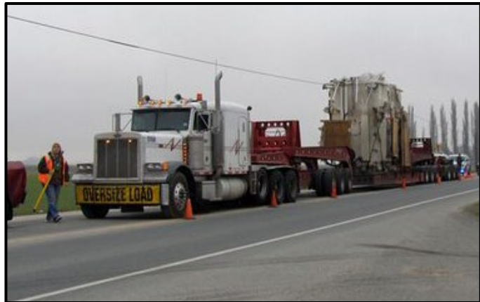
Super-load requiring bridge loading analysis.
