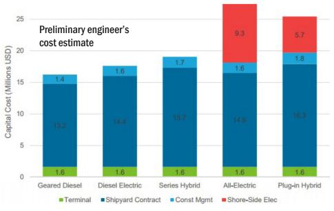
pulsion type; additional costs come into play for shoreside infrastructure, fuel and/or electric costs, and mid-life repowering, whether to an engine or for battery replacement.
