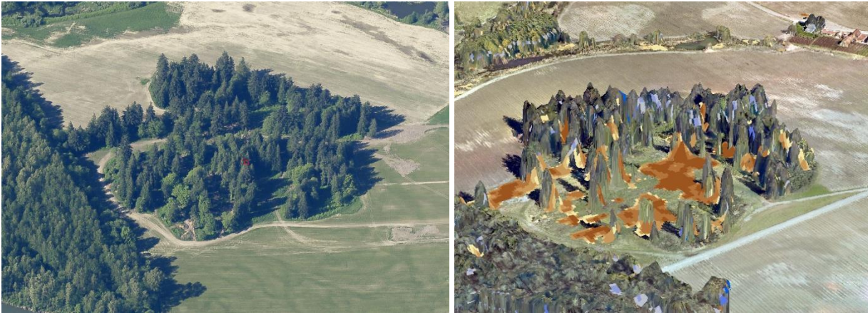
left: 2013 aerial photography of forest cover before clearing right: 3D model of same area based on 2015 photography; brown identifies lower height, indicating clearing
