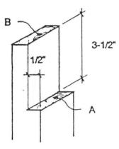
Connect each pair of frames together with two hinges. Then put the hook and eye gate latches on the other ends so that the sections latch together.
